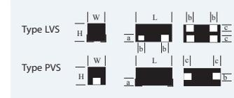
PRC's unique "single joint" design on the 4-tab LVS Series makes tab I.D. academic so you may select the pair closest to the top as your sense leads & the bottom pair for the current leads or vice versa
