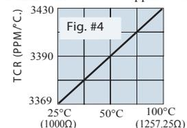
e.g. 1000Ω at 25°C. is 1257.25Ω at +100°C.
